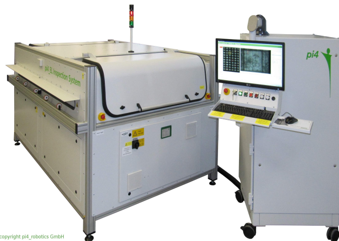
Automatic inline EL-inspection
