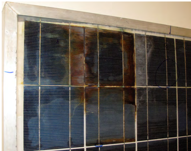
Fig. 4: Glass/glass module with specific ionomer encapsulant type that has proven to have insufficient adhesion, showing delamination and corrosion.
