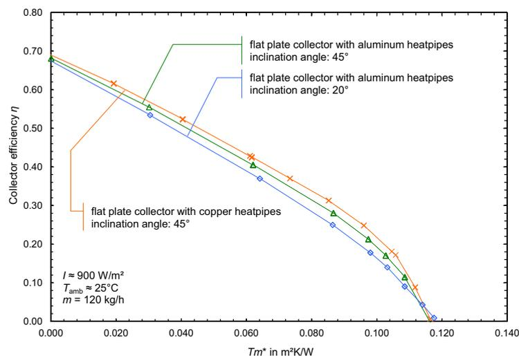
**Figure 7: Measured efficiency curves of novel flat-plate collector prototypes with reduced performance at high temperatures due to the use of deactivating heat pipes for different tube materials and inclination angles.**
