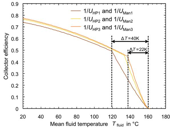
**Fig. 4:** Calculated influence of the thermal resistances of the heat pipe and the manifold on the collector efficiency and the shut down behaviour of a standard evacuated tube collector with an alkane as working fluid.
