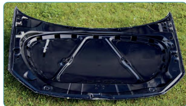
Left: Front side of a VIPV module based on a passenger car hood equipped with half-cut back contact solar cells resulting in a uniform color appearance. Right: its rear side with the supporting structure.
