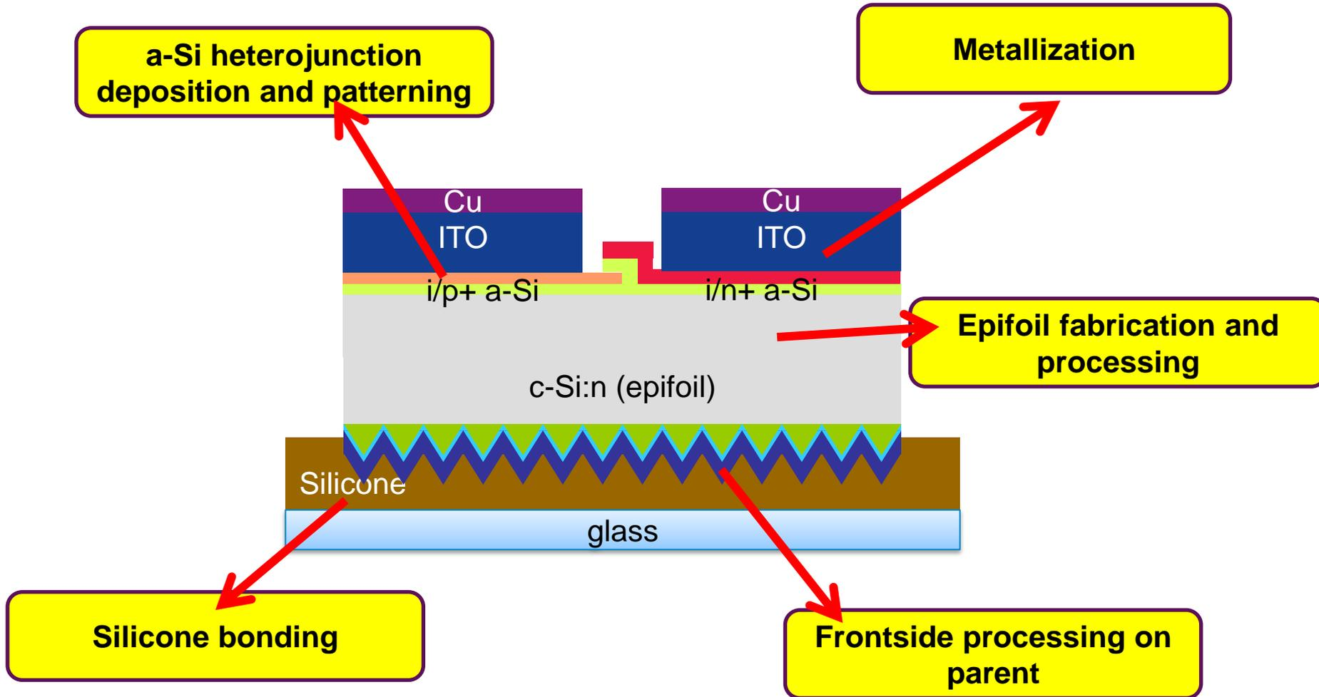
At device level: first simple devices of epifoils bonded to glass using silicones: **Voc values ~ 695 mV**
