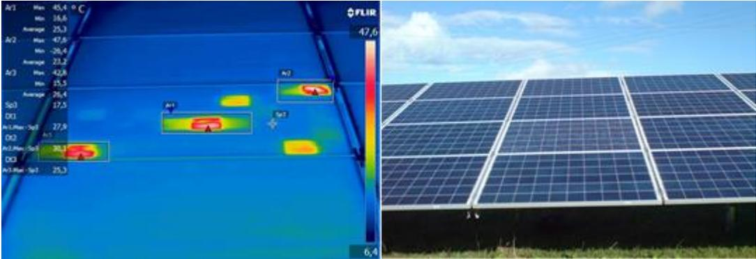
Figure 2-6: Breakage of front glass.
