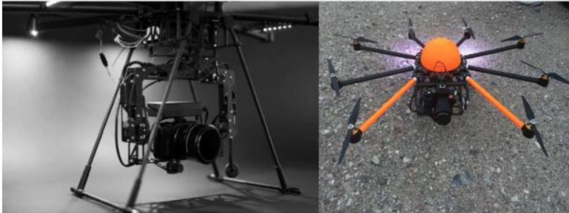
Figure 3-7: EL camera mounted on octocopter [79].
