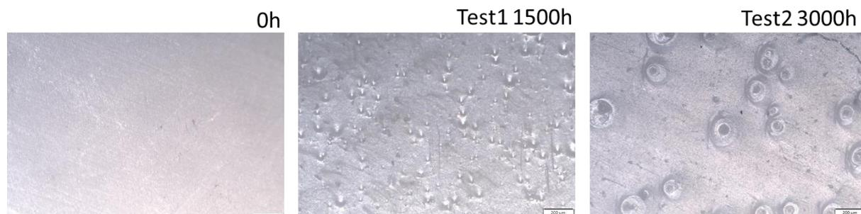
**Figure 22: Detached surface of the PO encapsulant from the glass in the original state 0 hours and after two types of accelerated ageing tests. Test1: constant Xe-irradiation at 1000 W/m<sup>2</sup> at elevated temperature (chamber 65°C, PV module 96°C) and humidity (80%r.H.). Test2: sequential (i) 500 hours DH, (ii) 50 temperature cycles and (iii) 200 hours Xe-irradiation at 1000 W/m<sup>2</sup>, 3 sequences.**
