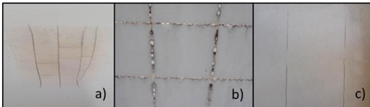
**Figure 19: Backsheet crack types. a) cracked backsheet beneath a hot cell/temperature induced crack. b) squared cracks beneath cell interspaces; thermo-mechanical induced crack combined with photo-oxidative degradation. c) longitudinal cracks located beneath busbars; thermo-mechanical stress induced crack [69].**
