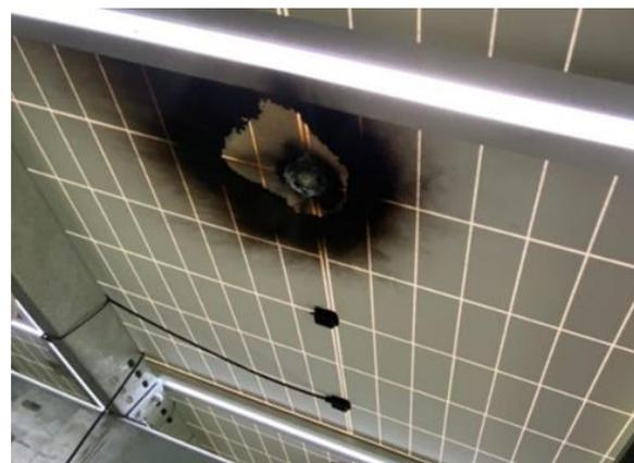
**Figure 18:** Module with burnt junction box resulting from unstable connection in the junction box.
